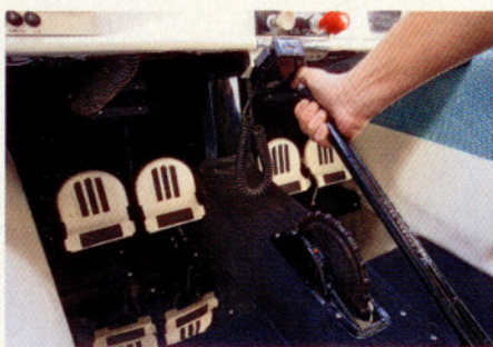
The standard arrangement ("six pack") of flight instruments (above) had yet to be adopted in 1956. Raising the lengthy handle (immediate left) lowers the large and effective flaps in 10-degree increments to a maximum of 40 degrees.
