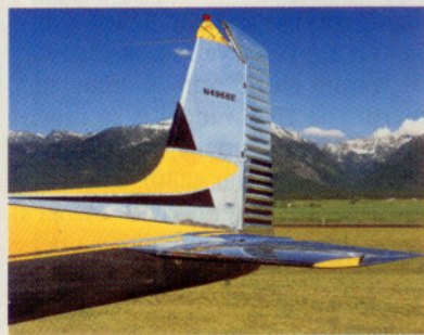
Original Cessna 182s were delivered with bare aluminum and trimmed in black and your choice of Pawnee yellow (above), scarlet, aqua, or Regal red. The baggage compartment (above, center) holds up to 120 pounds. Elevator trim utilizes an adjustable horizontal stabilizer (above).
