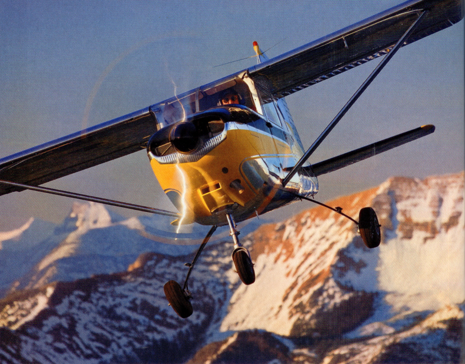
The first production Cessna 182 shows off over Montana's Glacier National Park. The long and spindly landing gear legs were shortened in subsequent models to make it easier to climb in and out of the cabin.
